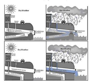
Figure E2-10 Example of a combined sewer system at the top and a separated sewer system at the bottom (Department for Environmental Protection, 2011<sup>viii</sup>)
