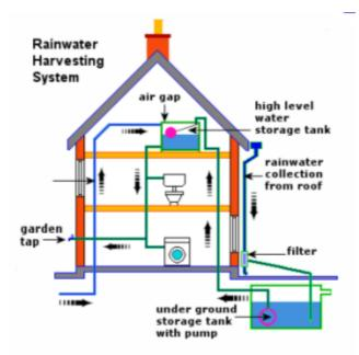
Figure E2-4 Example of a rainwater harvesting system (lowenergyhouse.com, 2011<sup>iv</sup>)
