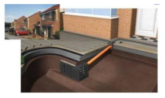
Figure E2-2 Example of a soakaway within a residential development (BCProfiles, 2011<sup>ii</sup>)
